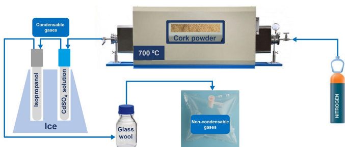
Fig. 3. Schematic representation of the experimental setup used to perform the pyrolysis of cork and collection system for handling condensable and non-condensable gas fractions.
