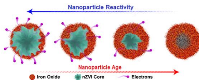
Fig. 8. Effect of aging on the reactivity of ZVI nanoparticles. Adapted and redrawn from Cecchin et al. (2017).
