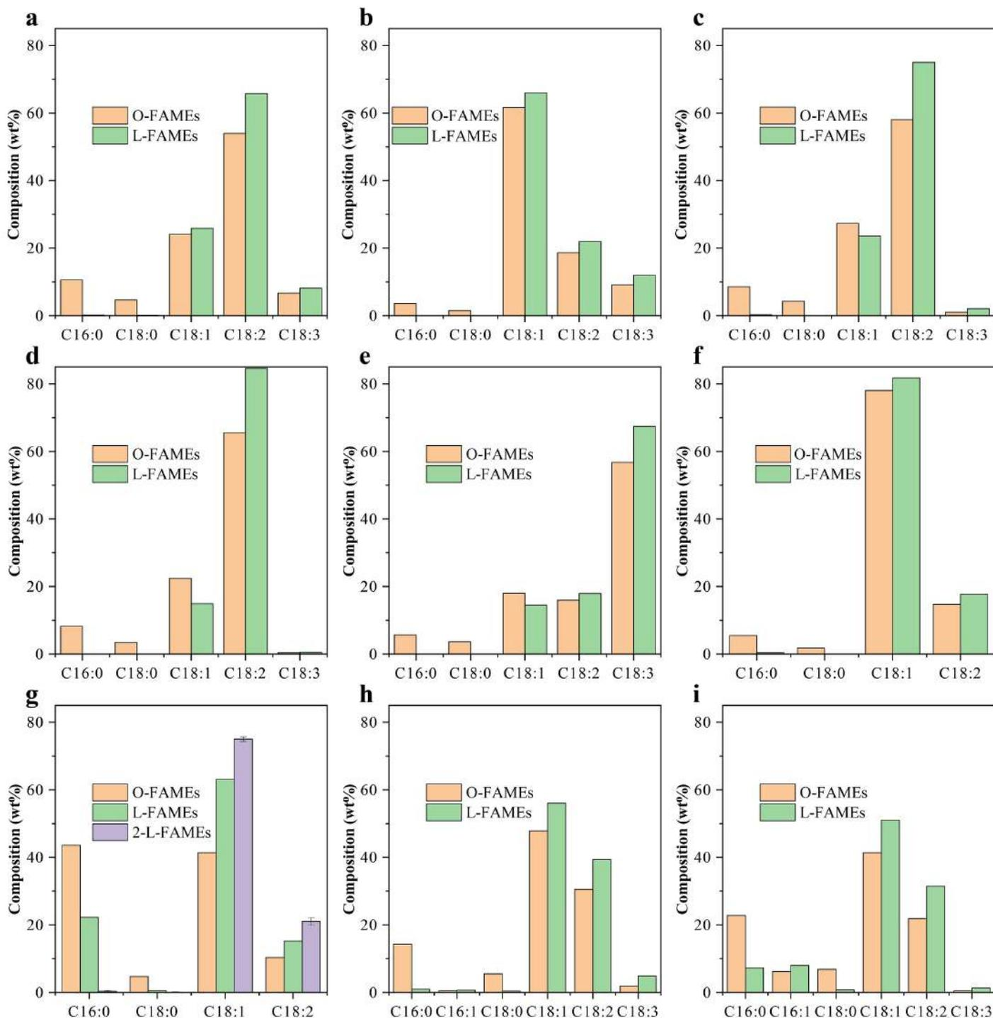
**Fig. 10.** Comparison of the original FAMES (O-FAMES) composition to L-FAMES after urea inclusion fractionation under the following operation conditions: FAMES (50 g), urea (50 g), methanol (200 g), and operating temperature of 0 °C: (a) soybean oil FAMES, (b) canola oil FAMES, (c) corn oil FAMES, (d) grape oil FAMES, (e) flaxseed oil FAMES, (f) high oleic safflower oil FAMES, (g) palm oil FAMES, (h) waste cooking oil FAMES, and (i) chicken fat FAMES.
