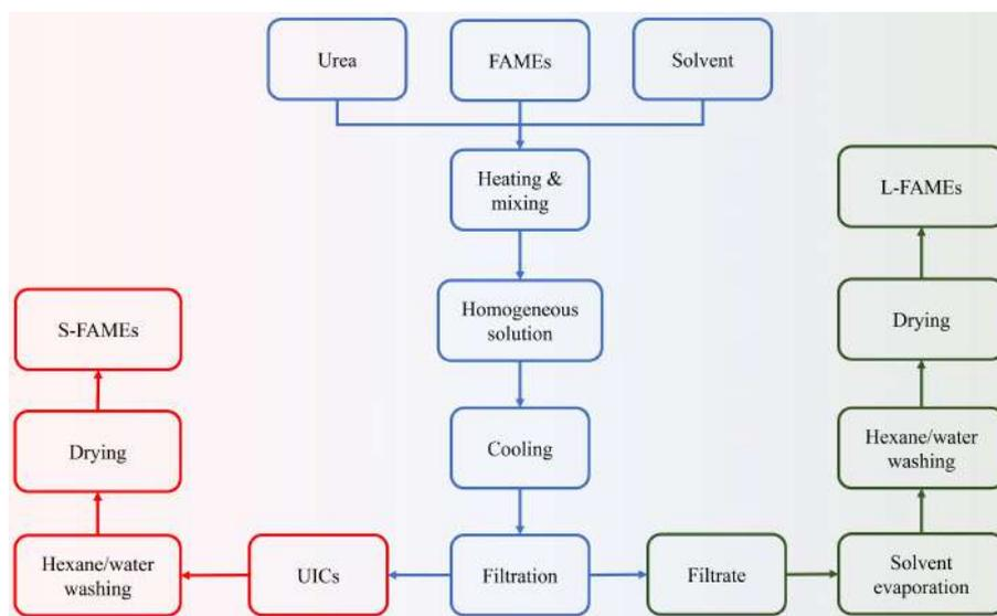
Fig. 2. Scheme of the cooling urea inclusion process.
