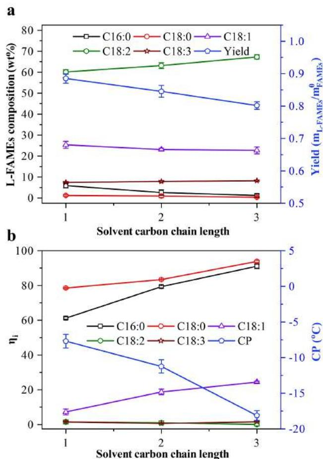
**Fig. 7.** Compositions, yields, and CPs of L-FAMES and separation efficiency ( $\eta$ ) of urea inclusion fractionation with various solvents (1: methanol; 2: ethanol; 3: n-propanol) under the operation conditions of soy FAMES (50 g), urea (30 g), solvent (200 g), and UIC formation temperature (0 °C) (a) composition and yield of L-FAMES, and (b) separation efficiency and CPs.
