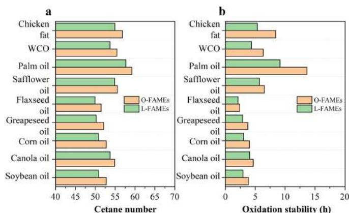
**Fig. 12.** Changes in cetane number and oxidation stability after urea inclusion fractionation under the operation conditions: FAMES (50 g), urea (50 g), methanol (200 g), and operating temperature of 0 °C. (a) cetane number and (b) oxidation stability of original FAMES (O-FAMES) and L-FAMES produced from different oil/fat feedstocks.
