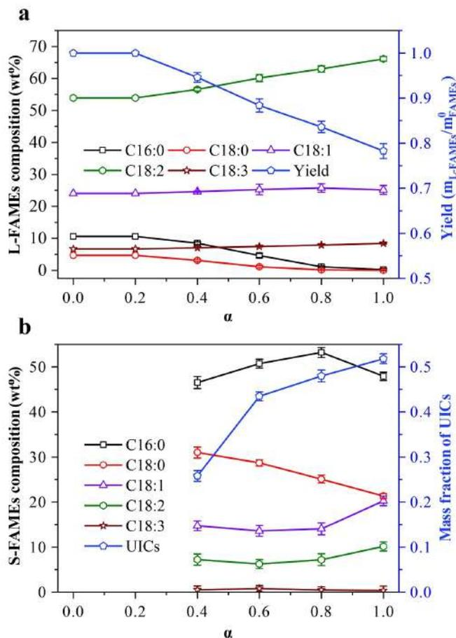
Fig. 3. Effect of mass ratio of urea to FAMES ( $\alpha$ ) on the compositions of FAMES in the liquid phase (L-FAMES) and FAMES in UICs (S-FAMES) (wt%), yields of L-FAMES, and UIC fraction under the processing conditions of soy FAMES (50 g), urea (0, 10, 20, 30, 40, and 50 g), methanol (200 g), and UIC formation temperature (0 °C); (a) compositions and yields of L-FAMES and (b) compositions of S-FAMES and mass fraction of UICs.
