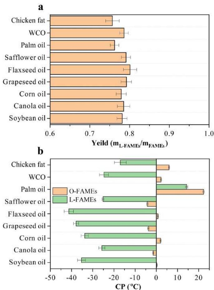
**Fig. 11.** Effect of urea inclusion fractionation on FAMES from various feedstocks under the processing conditions of FAMES (50 g), urea (50 g), methanol (200 g), and operating temperature of 0 °C. (a) yield of L-FAMES and (b) CPs of original FAMES (O-FAMES) and L-FAMES produced from different oil/fat feedstocks.
