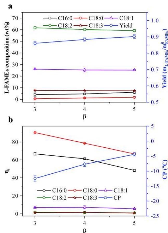
**Fig. 5.** Effect of mass ratio of methanol to FAMES ( $\beta$ ) on the composition of FAMES in the liquid phase (L-FAMES), separation efficiency ( $\eta_i$ ), yield, and CP under the processing conditions of soy FAMES (50 g), urea (30 g), methanol (150, 200, and 250 g), UIC formation temperature ( $0^{\circ}\text{C}$ ) and various mass ratios of methanol to FAMES; (a) composition and yield of L-FAMES, and (b) separation efficiency and CP.
