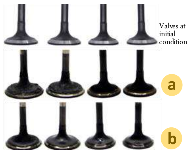
Fig. 12. Deposits formation on the cylinder 1 valves of the vehicles powered by (a) B40 and (b) B30D10 after the 50,000 km endurance test.
